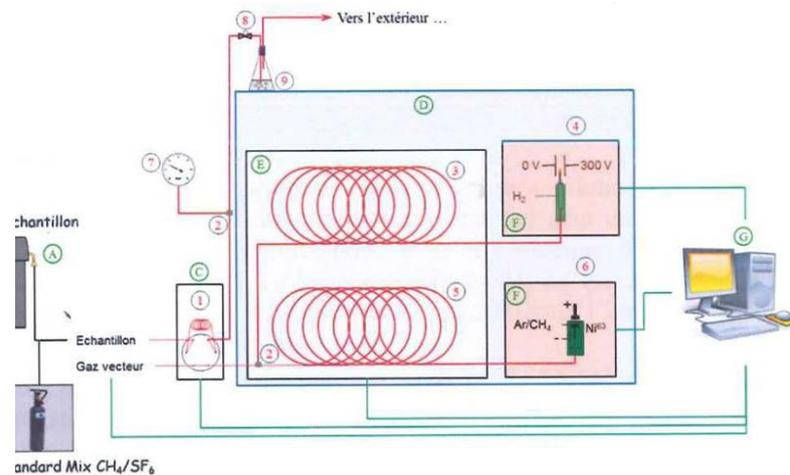
Fig. 3: Schematic representation of the GC
