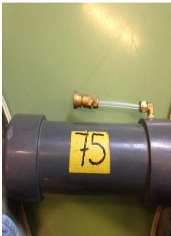
Fig. 2: Evacuated canister
