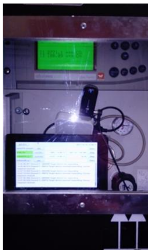
Photos 5, 6. Infrared spectroscopy analyzers SERVOMEX 4100 on the farms
