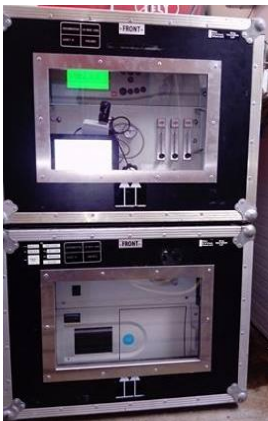
Photos 5, 6. Infrared spectroscopy analyzers SERVOMEX 4100 on the farms
